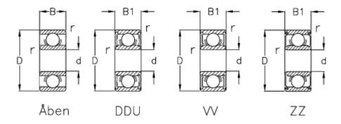
Max rpm ZZ-WW = 36000 В = 6 B1 = 6 r min = 0.3= 7 Type = 607 d D = 19 Load Cor (N) = 885Load Cr (N) = 2340Max rpm DD = 32000Max rpm open = 43000
